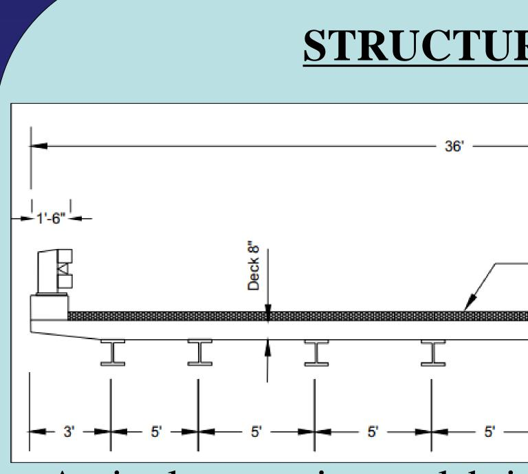
A single span integral brid abutments will be used for For this design, the use c will be implemented along 10m steel railing. The deck by seven steel girders wearing surface of the deck an epoxy overlay. An generally less expensive and maintenance.
