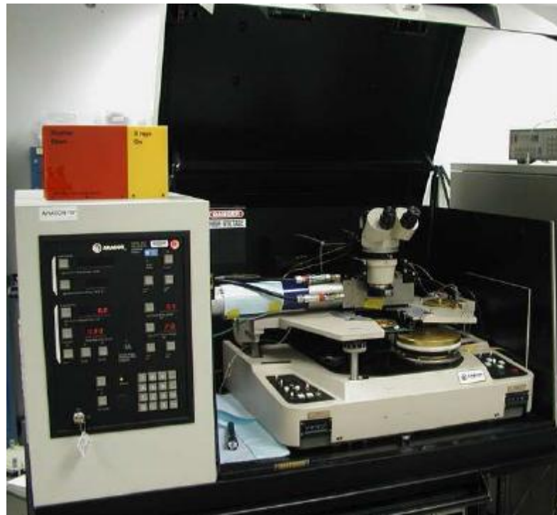
Figure 5.1: Image of an Aracor 4100 Wafer-Level X-ray Irradiator (17).
