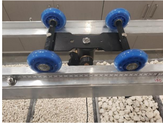
Figure 2. Rail system and trolley for mounting imaging equipment.
