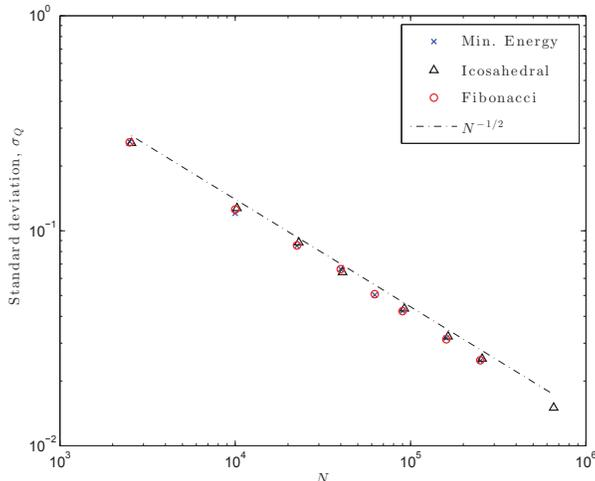
Figure 2: Estimate of the standard deviation  $\sigma_Q$  in (2.17) for the different families of nodes. The estimate is based on sample sets of 500  $N$ -point quadratures of different independent, identically, distributed, zero mean (quasi) random data with a standard deviation of 1. The dashed line corresponds to taking all weights equal in (2.17), which gives  $\sigma_Q = 4\pi\sigma_\nu N^{-1/2}$ . This confirms the stability estimate in the last part of Theorem 4.10.
