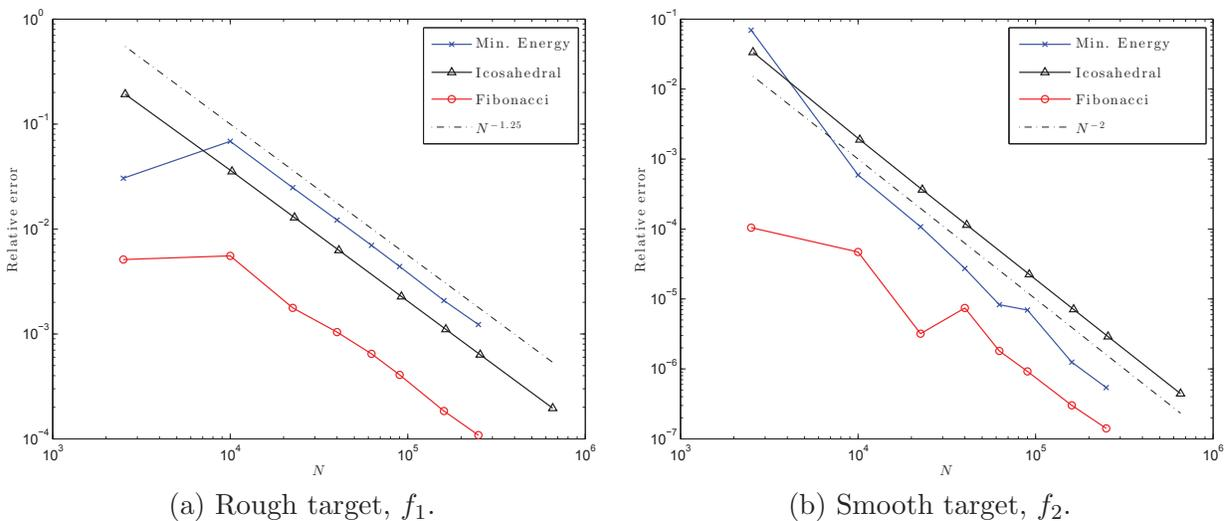
Figure 4: Relative errors in the  $N$ -point quadratures of (a)  $f_1$  and (b)  $f_2$  for the three different families of nodes. The mesh-norm for all three families of nodes satisfies  $h \sim N^{-1/2}$ , so that the dashed lines in the figures indicate convergence like (a)  $\mathcal{O}(h^{2.5})$  and (b)  $\mathcal{O}(h^4)$ . These are the predicted convergence rates from Theorem 4.10 and Corollary 4.11, respectively.
