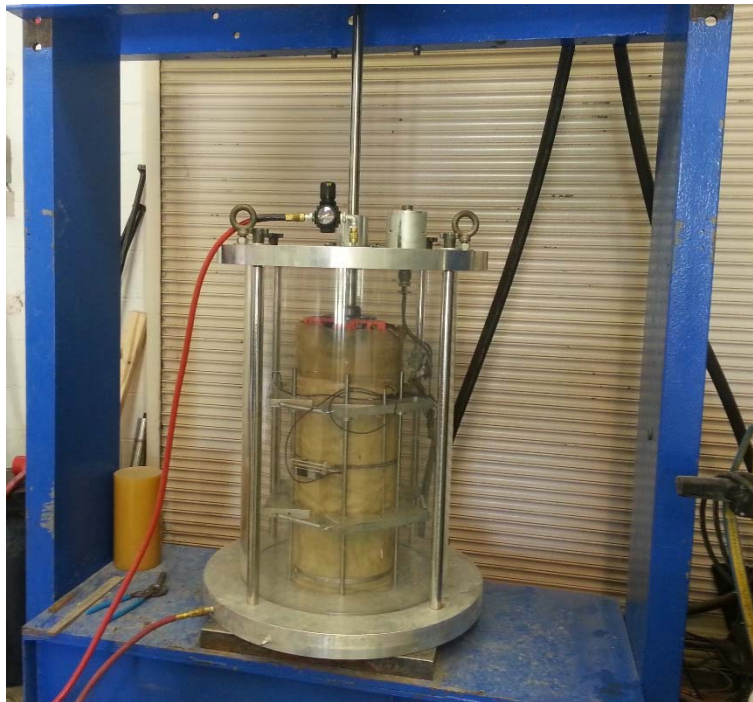
FIG. 1. The University of Illinois ballast triaxial tester (TX-24)
