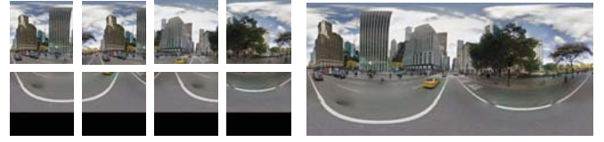
(a) Small images with level 2 quality (b) Panoramic photo stitched from the small images
