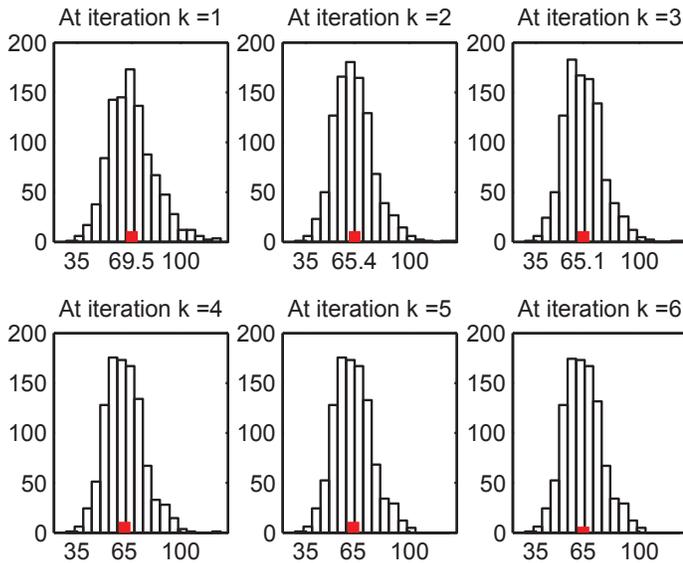
FIG. 3. Histogram showing the sample distribution of  $\tilde{\mathcal{J}}_k(\mathbf{x})$  at each Gauss–Newton iteration for the cross-well tomography problem. The mean of the sample is shown as the middle red tick.
