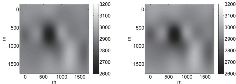
FIG. 7. Solutions found for the tomography problem with  $\mathbf{L}$  discrete approximation to the Laplacian. Left: Solution found using the discrepancy principle. Right: Solution found with Algorithm 1.
