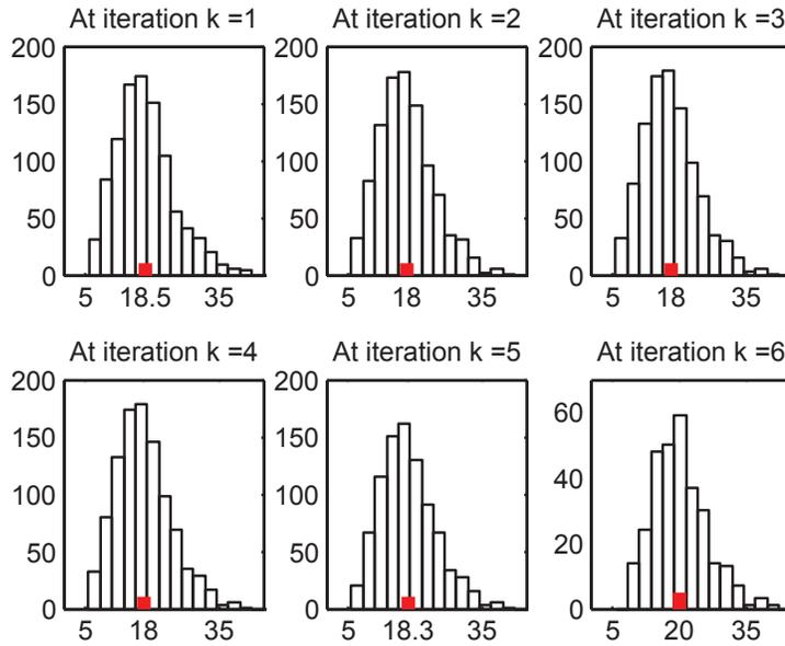
FIG. 5. Histograms of  $\tilde{J}_k^{LM}(\mathbf{x})$  at each Levenberg–Marquardt iteration for the electrical conductivities problem.  $C_f = \sigma_f^2 \mathbf{I}$ . The sample mean is shown as the middle tick.
