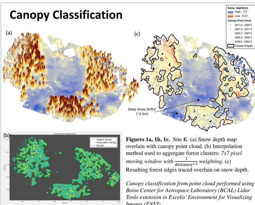
**Figures 1a, 1b, 1c.** Site K (a) Snow depth map overlain with canopy point cloud. (b) Interpolation method used to aggregate forest clusters: 7x7 pixel moving window with  $\frac{1}{\text{distance}^{1.2}}$  weighting. (c) Resulting forest edges traced overlain on snow depth.
