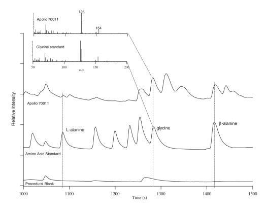
Fig. 2. GC–MS/IRMS analysis of the derivatized extracts from Apollo 70011 and of an amino acid standard and procedural blank. The traces show the m/z 44 ( ${}^{12}CO_2$ ) peaks produced during GC-IRMS analysis. The inset shows the simultaneously collected mass spectral fragmentation pattern for the peak assigned to glycine in the Apollo sample and the standard, which indicate minimal contributions from non-glycine coelutions.
