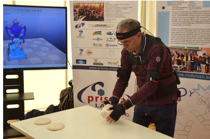
Fig. 7: The renowned pizza chef Enzo Coccia wearing the Xsens MVN suite, with the RODYMAN avatar in the background acquiring and repeating the movements of the chef.
