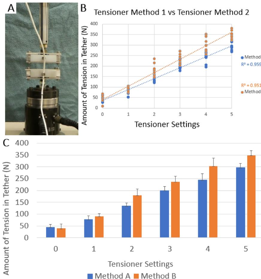
Figure 2: (A) mechanical fixture (B,C) Tension [N] at each tensioner setting for both methods
