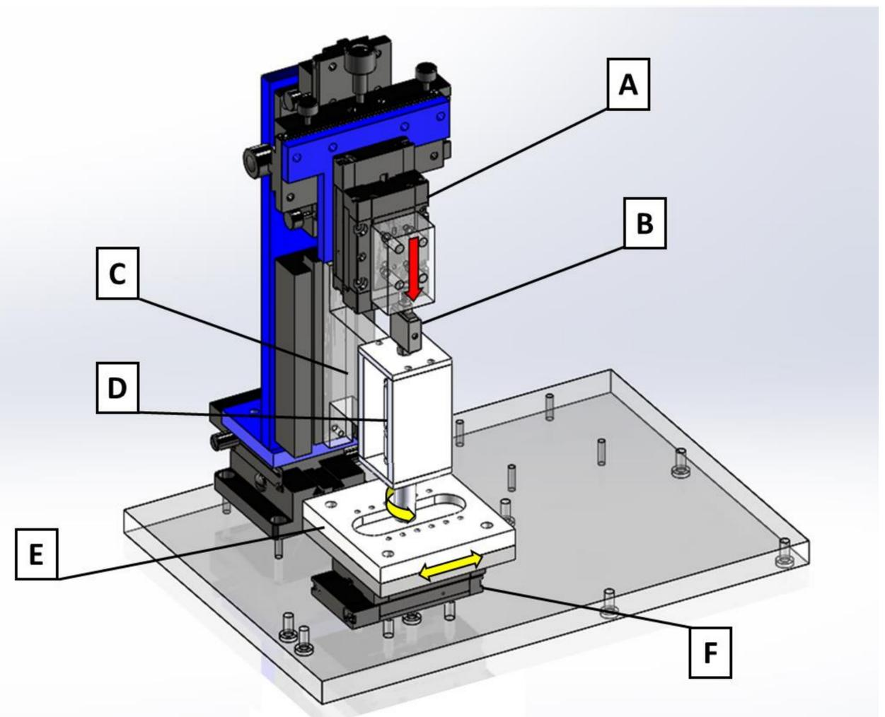
Figure 3: 3D model of the POD design with rotations + translations and axial force shown.
