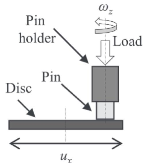
Figure 2: Schematic of the proposed pin-on-disk fixture. Motions include the horizontal translation of the disk and the axial rotation of the pin<sup>3</sup>
