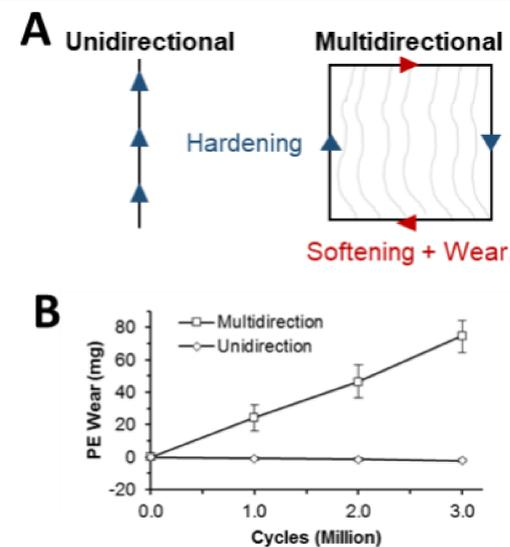
Figure 1: A) Schematic of multidirectional loading and B) Polyethylene wear
