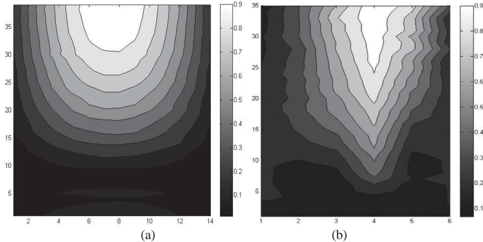
**FIG. 4. Normalized electric-field contour-map: (a) simulation; and (b) experimental measurements. The contourmaps are plotted on a depth (vertical) slice located 2 cm from the center of the box toward the antenna.**
