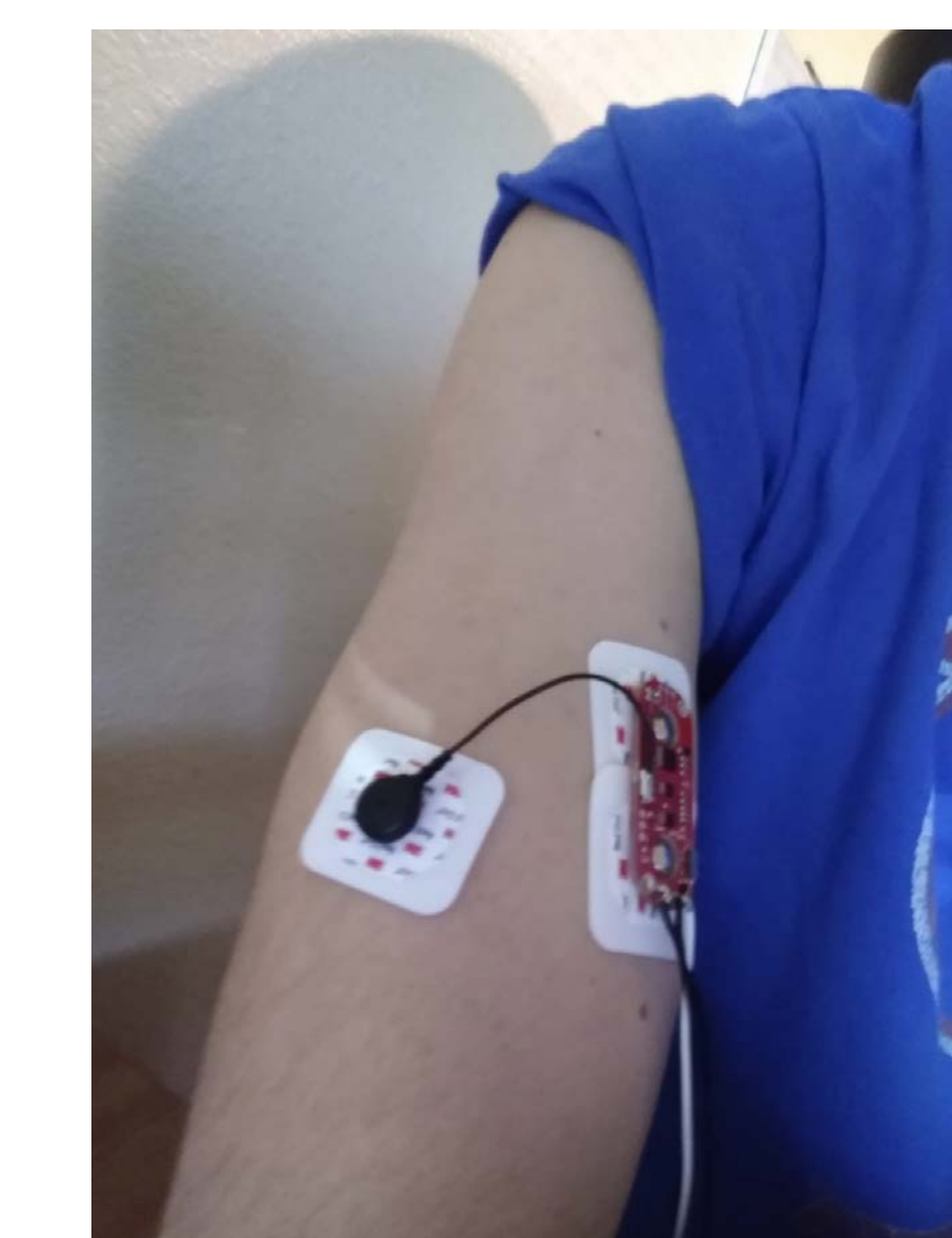
Figure 10 - Myoelectric sensor attached to upper arm
