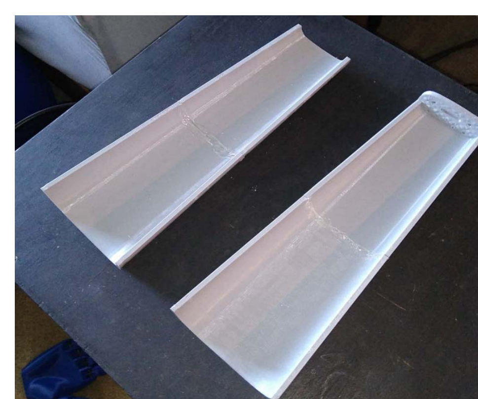
Figure 3 - 3D printed forearm split into two parts, first design iteration, electronic components and a battery will be stored in here
