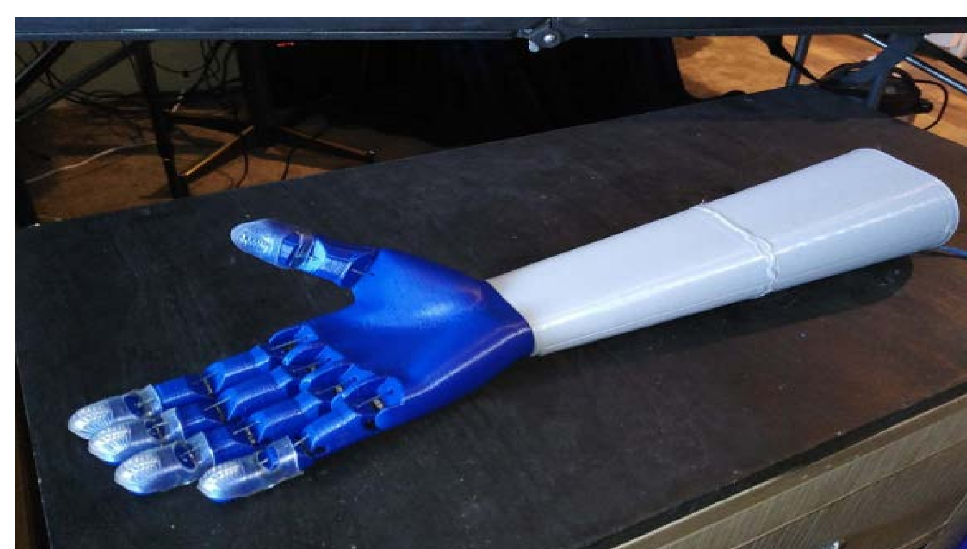
Figure 5 - 3D printed forearm and hand put together
