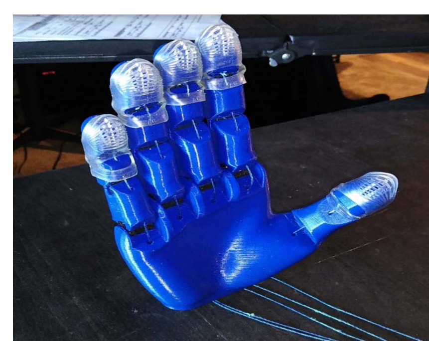
Figure 2 - 3D printed Flexy-Hand designed by Gyrobot
