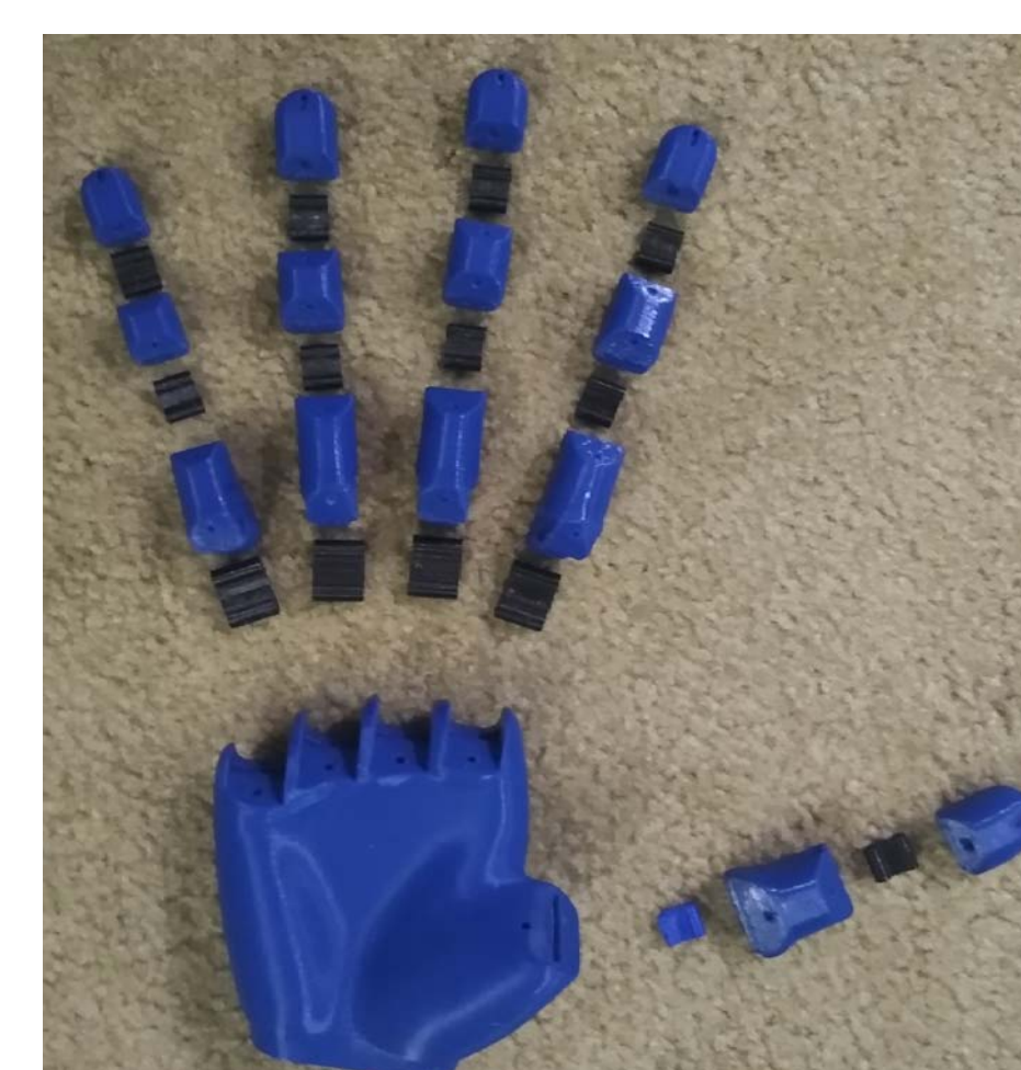
Figure 4 - 3D printed Flexy-Hand designed by Gyrobot in exploded view
