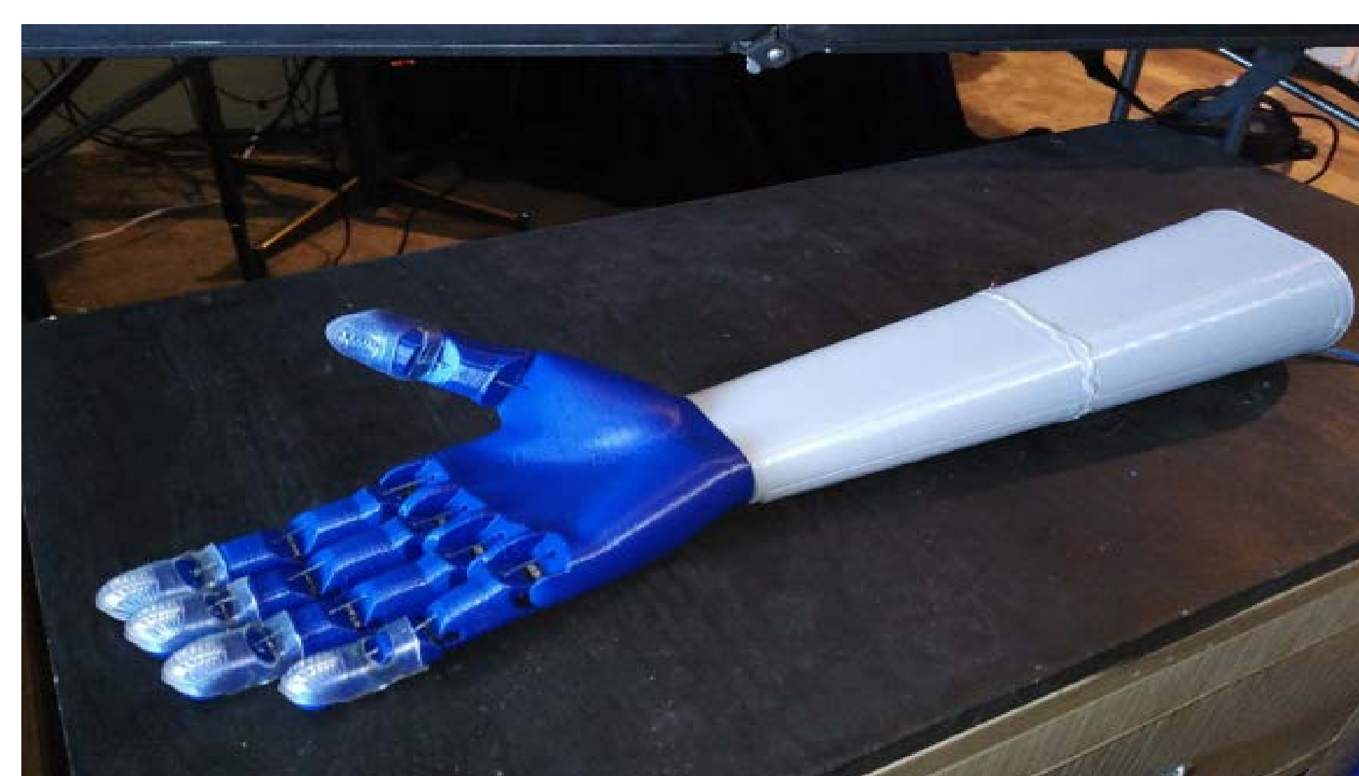
Figure 5 - 3D printed forearm and hand put together
