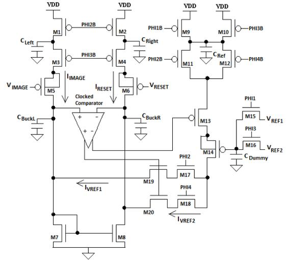
Figure 3. DSM ADC with gain error correction circuitry.
