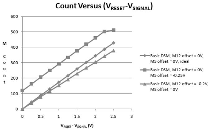
Figure 6. Simulation results for the DSM without offset and gain error correction. Different voltage offsets are applied to M5 and M12.
