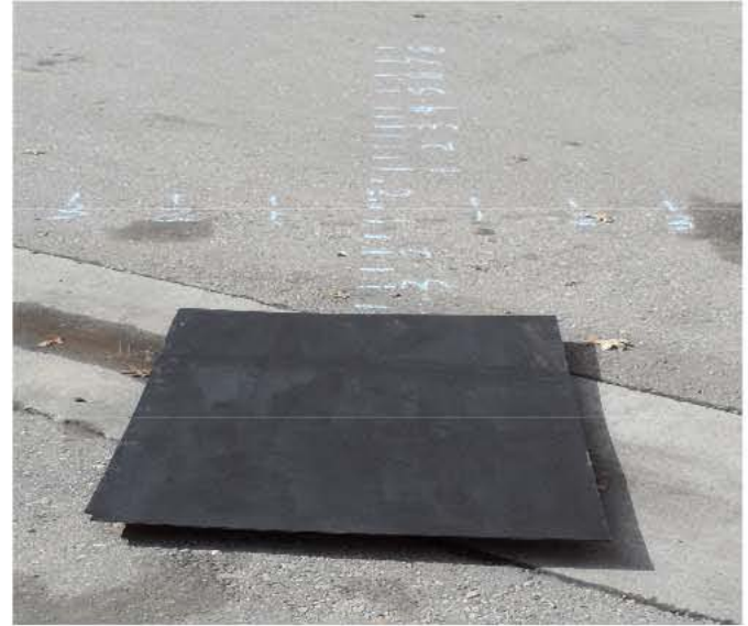
Figure 3. Insulation Board for Temperature Measurement in the Field
