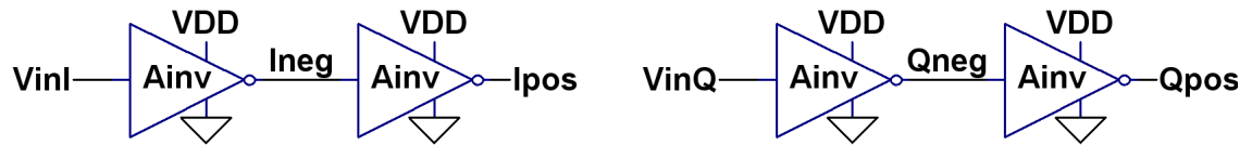
Figure 27. Inverters used to generate four phases from the two quadrature phases.
