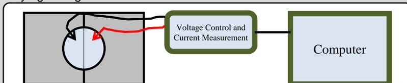
Figure 2. Setup to measure conductance across a lipid bilayer
