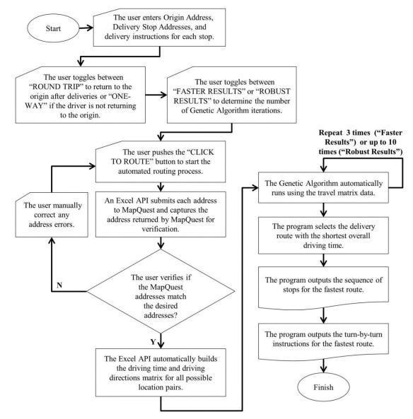
Figure 1: The flowchart describes the operation of the routing tool we developed.
