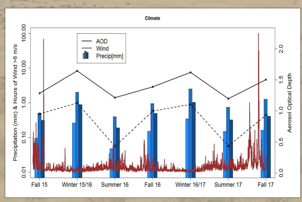
Wind above 6m/s is needed to entrain particles but precipitation is also necessary to effectively remove the particles from the atmosphere. The data above is normalized by the number of days in a sampling interval showing that the fall is both windier and wetter per day than summer.
