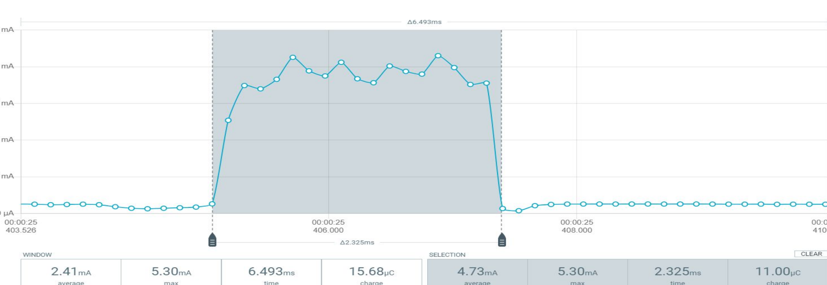
Figure 7: A zoomed-in view of the current draw while encrypting one message with Ascon
