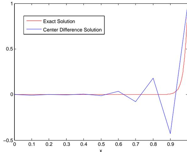
Figure 2.2: Oscillations present using central difference for  $\beta > 2$
