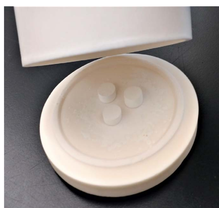
Figure 7 : Inverted crucible with sintered pellets
