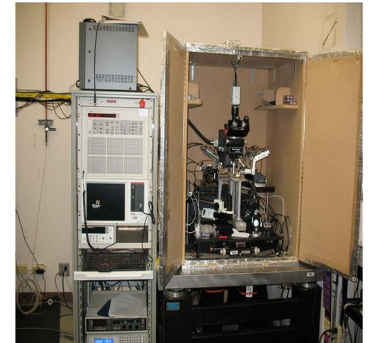
Fig. 7 Keithly characterization system used to perform voltage sweep test on devices
