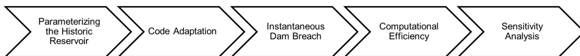
Figure 2.3: The workflow to develop the GeoClaw Teton Dam model consisted of five primary steps: (1) parameterizing the historic reservoir, (2) adapting the code, (3) parameterizing an instantaneous dam breach, (4) maximizing computational efficiency, and (5) performing a sensitivity analysis for model uncertainties.
