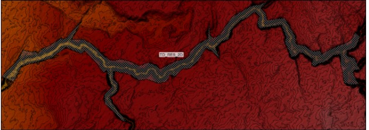
Figure A.10: 2D Teton Reservoir flow area constructed using dx=200 ft, dy=200 ft. Labeled TDRES2D.
