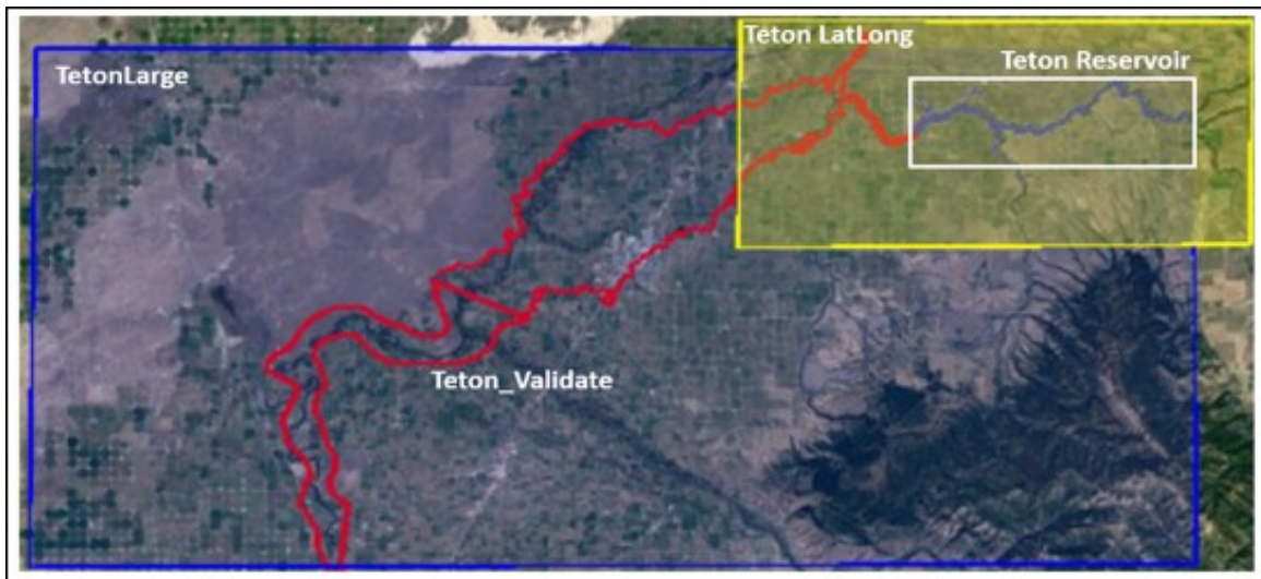
Figure 2.1: TetonLarge and Teton LatLong DEM's along with the detailed Teton Reservoir and the red outline of the historic flood (TetonValidate). The domain extent above is 55 miles base by 27 miles length (88.5 km x 43.5 km).
