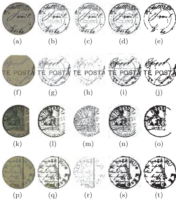
Figure 4: Postmark stamps (a) original, (b) general enhancement, (c) Sauvola from red and green planes, (d) combination of first enhancement and Sauvola, and (e) the “cleaned” postmark images omitting isolated text.
