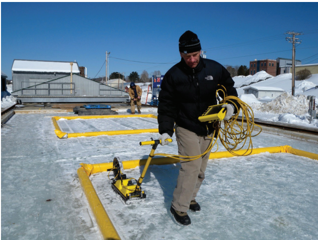
Figure 2. Photograph of the first author acquiring data along the tank axis with the 500-MHz antenna set. The antennas are inside the containment hoop with oil under the ice.
