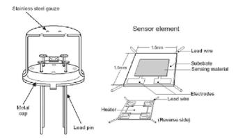
Figure 4. Metal Oxide Semiconductor Sensor Structure<sup>5</sup>.
