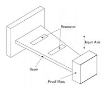
Figure 10. Surface Acoustic Wave Accelerometer<sup>11</sup>.
