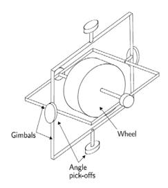
Figure 14. Mechanical Gyroscope<sup>11</sup>.
