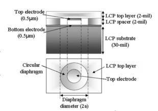
Figure 7. Capacitive Pressure Sensor9.
