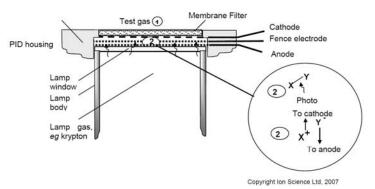
Figure 3. Photo-Ionization Detection (PID) Structure<sup>4</sup>.
