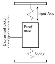
Figure 9. Mechanical Accelerometer<sup>11</sup>.
