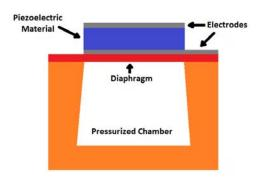
Figure 8. Piezoelectric Pressure Sensor.
