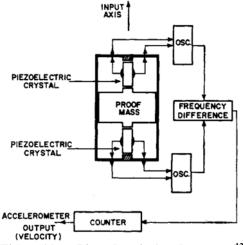
Figure 11. Piezoelectric Accelerometer<sup>12</sup>.
