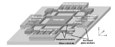
Figure 17. MEMs Gyroscope <sup>14</sup>
