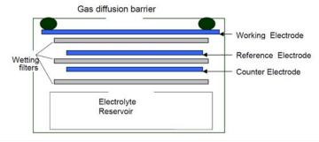
Figure 1. Electrochemical Chemical Sensor <sup>1</sup>.
