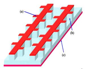
Figure 6. Polyimide Capacitive Humidity Sensor<sup>8</sup>.
