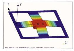
Figure 12. Trampoline type MEMs Accelerometer structure<sup>13</sup>.
