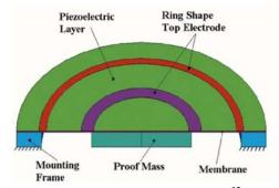
Figure 13. MEMs Accelerometer<sup>13</sup>.
