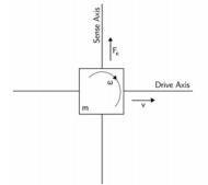
Figure 16. Coriolis Principle <sup>11</sup>.
