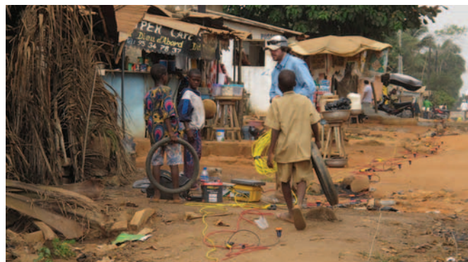
Figure 7. This photo shows a typical roadway used in acquisition. Limited access required that seismic lines be placed among small roadside businesses and homes. Heavy foot and vehicle traffic produced substantial coherent seismic noise. After Bradford and Lindsay, 2013, Figure 3.
