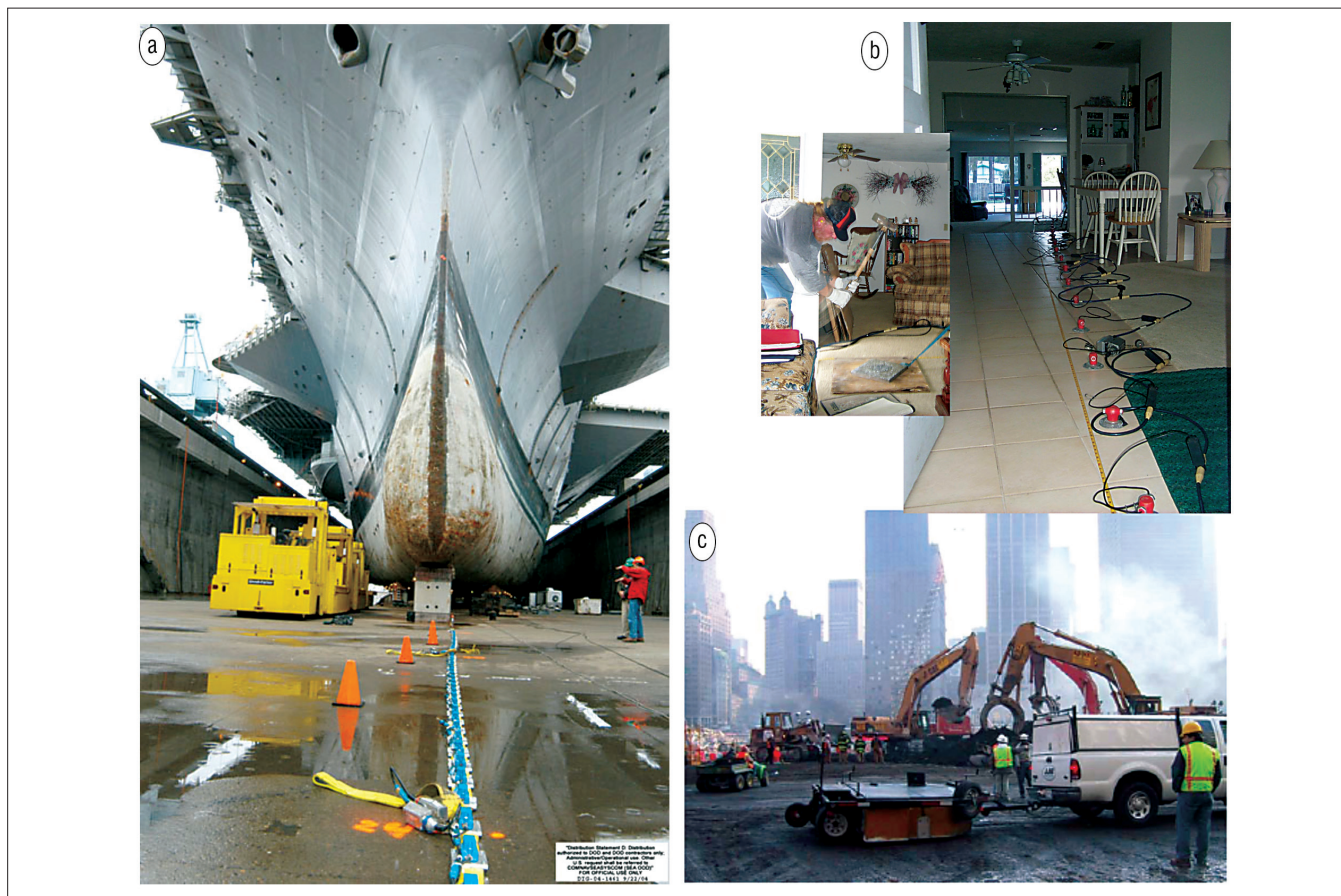
Figure 1. Geophysical data acquired in difficult settings: (a) seismic reflection data acquired in a shipyard (John Clark, personal communication), (b) MASW seismic data acquired through a house (Miller et al., 2000), and (c) radar acquisition in New York (Birken et al., 2002).
