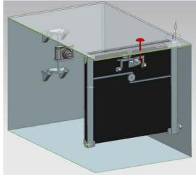
Figure 7. Mechanical design of Portable Ballot Counter.
