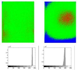
Figure 5. Left: Gray level contours for a uniformly colored document taken with the Epson Perfection 3170 Photo scanner. The highlighted levels are <220 (blue), 220-230 (green), and >230 (red); Right: Gray level contours for the same document taken with the Canon camera. The highlighted levels are <190 (blue), 190-200 (green), and >200 (red).
