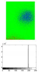
Figure 6. The iso-intensity contour level of the image in figure 5 after linear flattening. The highlighted levels are <194 (blue), 194-197 (green), and >197 (red), which is nearly a tenfold improvement over Figure 5.
