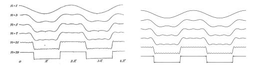
Fig. 9. On the left, a figure from Runge's 1904 book Theorie und Praxis der Reihen [25]. On the right, the equivalent computed with periodic Chebfun. Among other things, this figure illustrates that a trigfun can be accurately evaluated outside its interval of definition.
