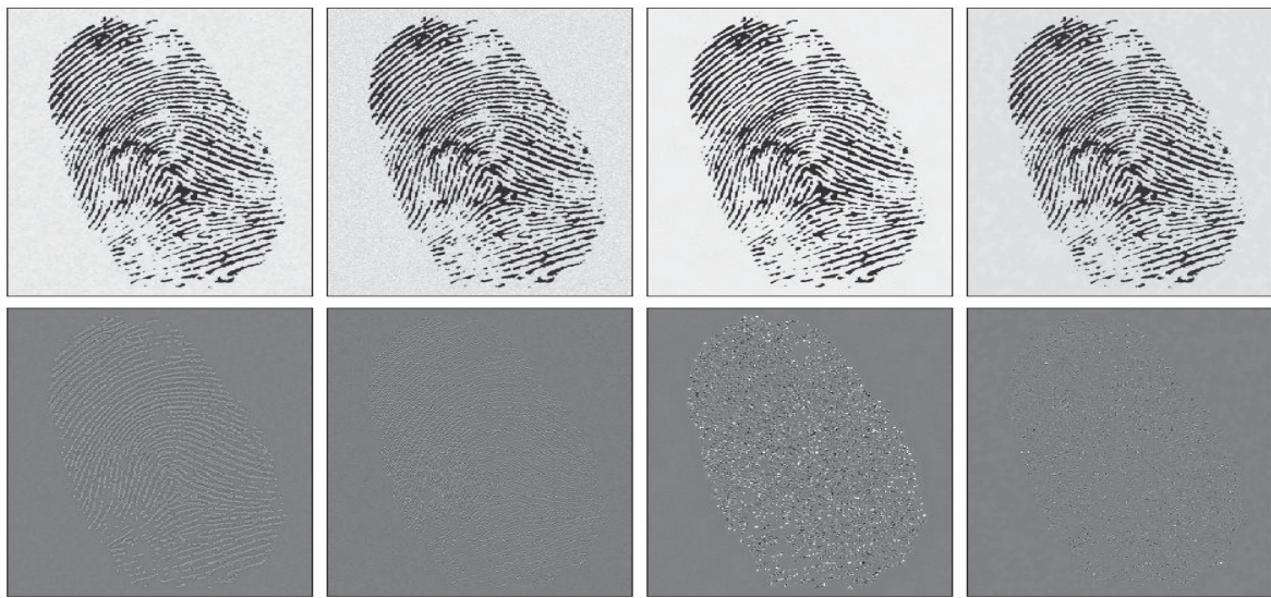
Figure 5: The first row shows the denoised fingerprint images by TV, ASSK, ONLM and NEW when \sigma = 10 . The second row shows their mean deviation images.
