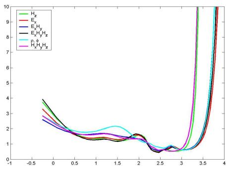
**Figure 5:** Spread computed from the PSFs obtained at the final iteration of the inversion. The x-axis is the depth plotted in the log scale i.e.  $log_{10}(z (m))$ .
