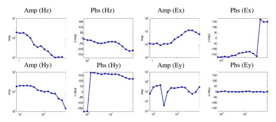
**Figure 1:** The  $\log_{10}(\text{amplitude})$  ( $\mu\text{V/m}$  for E and  $\mu\text{H/m}$  for H) and phase in degrees for multi-component CSAMT data as a function of  $\log_{10}(\text{frequency})$  in the range of 0.5-8192 Hz.
