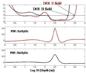
**Figure 6:** The top panel shows the spread function for the ExHyHz and HxHyHz field inversion. The level set indicated by the horizontal line indicates an iso-spread value chosen to examine the depth of investigation (DOI) of the fields. The middle and bottom panels are the PSFs of the conductive layer.
