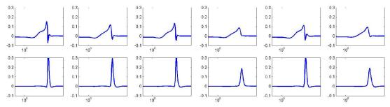
**Figure 4:** Averaging kernels obtained by inverting different components of the field individually or in combination (order is same as in Figure 3). The top panel shows the averaging kernels for the resistive layer. The bottom panel shows the averaging kernels for the conductive layer.
