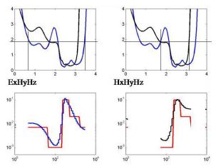
**Figure 7:** The top left and right panel shows the spread curves for the ExHyHz (blue) and HxHyHz (black). The level set for the spread value is shown by the black horizontal line. The vertical line on the spread plot shows the depth interval resolved by the data. The bottom left and right panels show the region of the model that is resolved by the available data.
