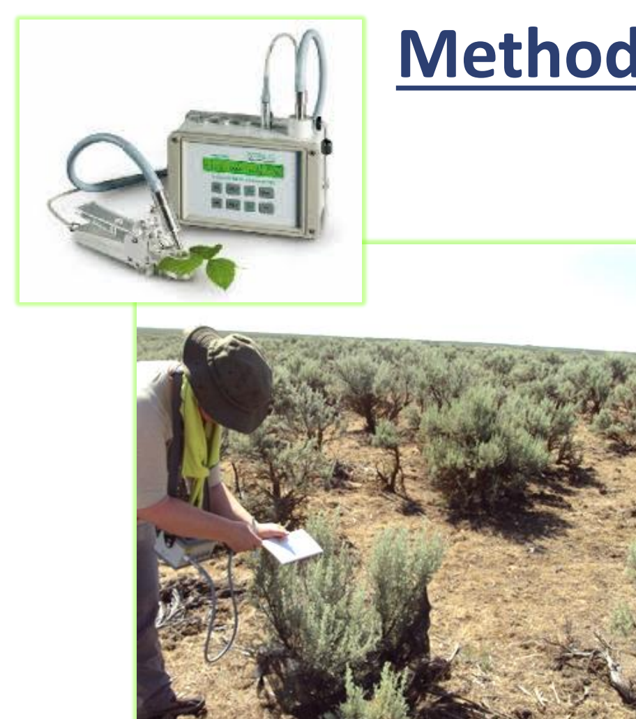
Figure 2. Using the fluorometer in the field. Measured three shrubs/site biweekly.
