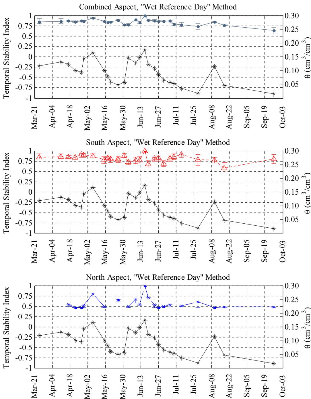
**Figure C3: The Temporal Stability Index Results for the “Wet Reference Day” method of calculation, the transect average soil moisture conditions are plotted in black for reference. All correlations are significant at  $p < 0.05$ ; error bars represent the range of values obtained by calculating the correlation coefficient from the results of Bootstrap resampling of soil moisture data.**
