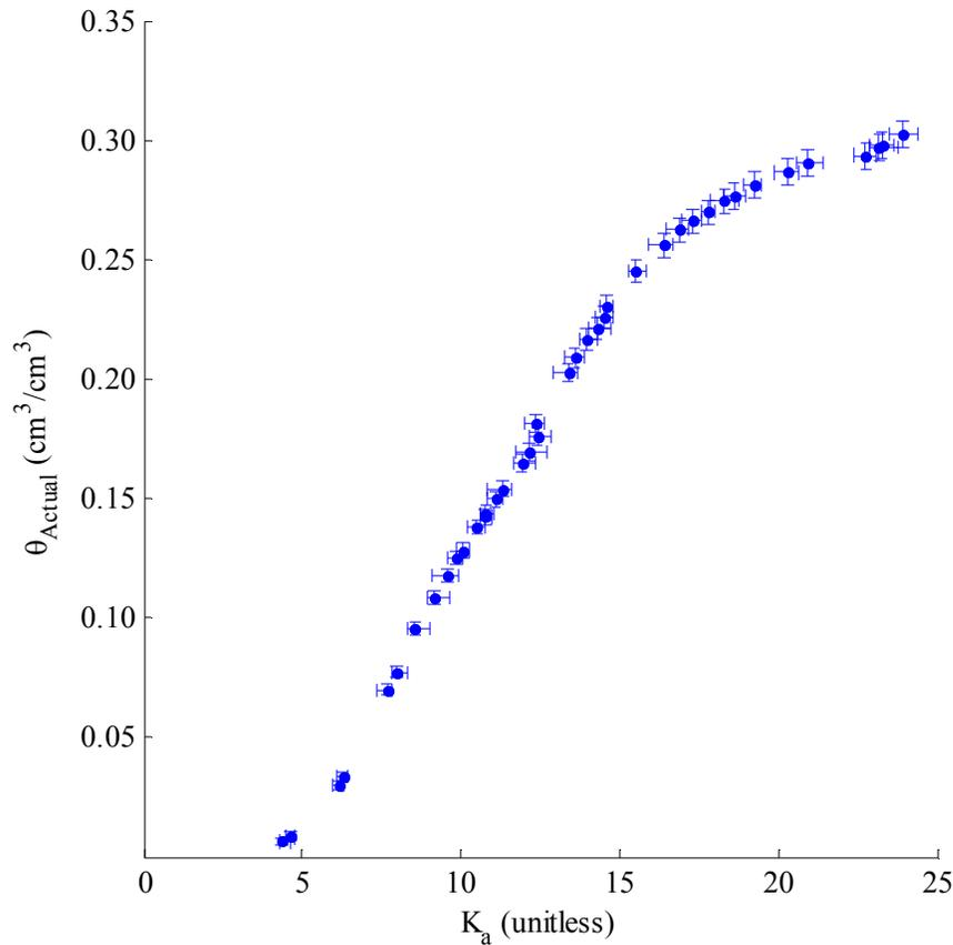
**Figure 2.1:  $\theta$  versus  $K_a$  for the TDR system calibration. Vertical error bars encompass the absolute uncertainty in the calculation of  $\theta$  in the calibration bucket. Horizontal error bars encompass the variation in  $K_a$  values at a given  $\theta$ .**
