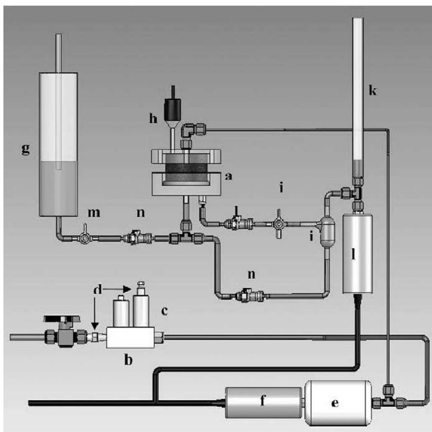
**Figure 2.3: Schematic of the automated multistep outflow setup for each cell: (a) Tempe cell, (b) aluminum mounting block, (c) Tempe cell, (d) orifices, (e) N<sub>2</sub> storage, (f) pressure transducer, (g) Mariotte bottle for saturating the sample, (h) pressure transducer, (i) fourway valve, (j) bubble trap, (k) burette, (l) pressure transducer, (m) clamp valve, (n) quick-disconnect valve. Image and description from Figueras and Gribb (2009).**
