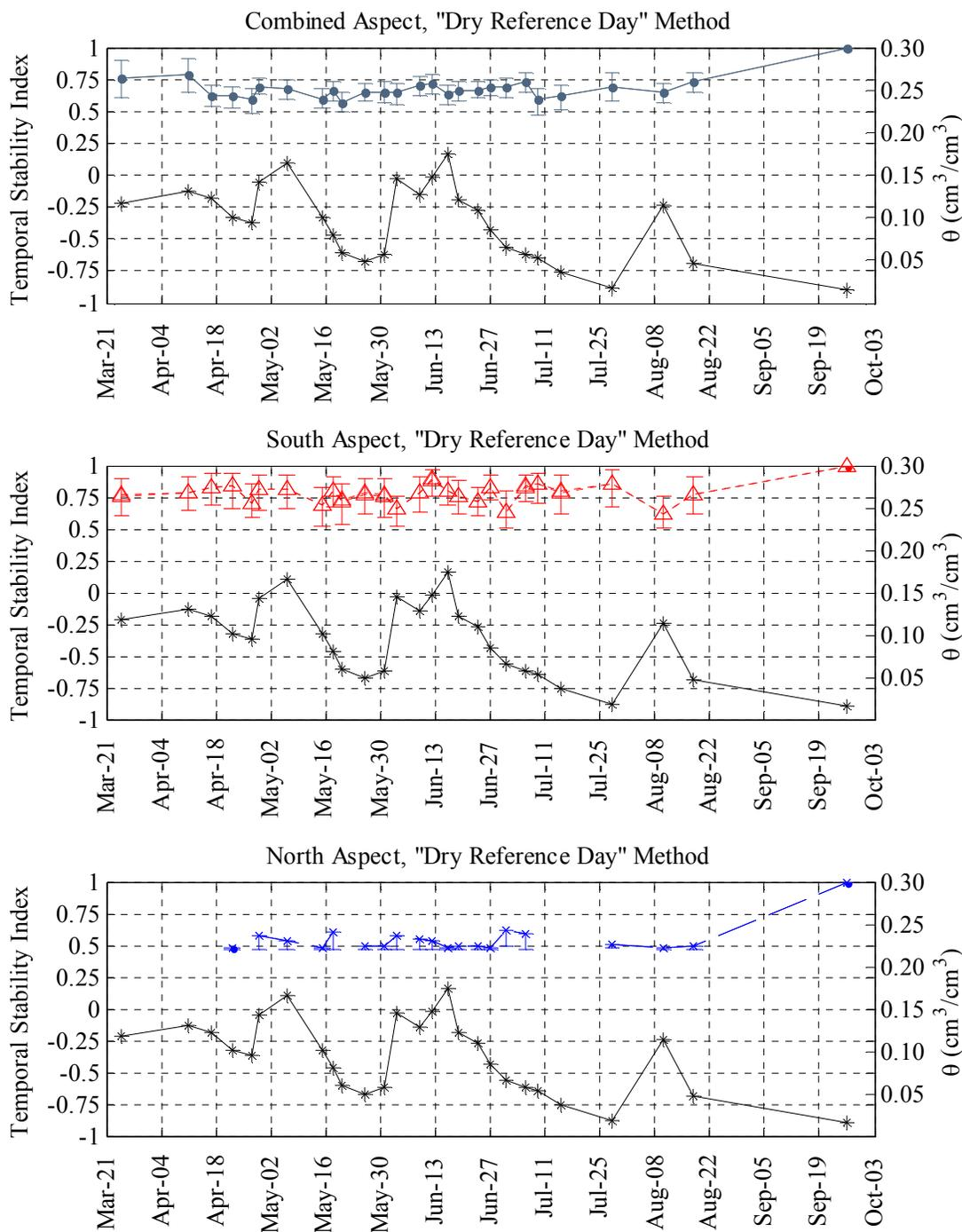
**Figure C2: The Temporal Stability Index Results for the “Dry Reference Day” method of calculation, the transect average soil moisture conditions are plotted in black for reference. All correlations are significant at  $p < 0.05$ ; error bars represent the range of values obtained by calculating the correlation coefficient from the results of Bootstrap resampling of soil moisture data.**
