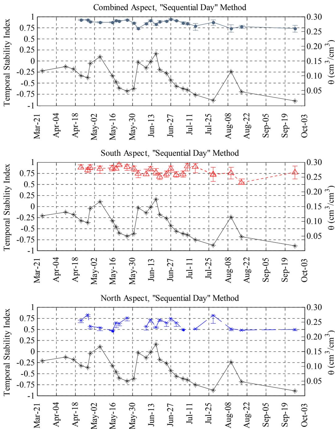
**Figure C1: The Temporal Stability Index Results for the “Sequential Day” method of calculation, the transect average soil moisture conditions are plotted in black for reference. All correlations are significant at  $p < 0.05$ ; error bars represent the range of values obtained by calculating the correlation coefficient from the results of Bootstrap resampling of soil moisture data.**
