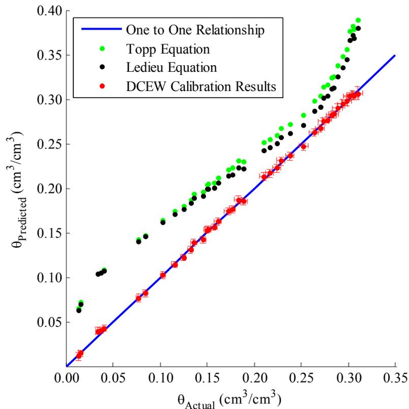
**Figure 2.2: Comparison of  $\theta_{\text{Actual}}$  versus  $\theta_{\text{Predicted}}$  for the TDR validation, as compared to the Topp et al. (1980) and Ledieu et al. (1986) equations. Horizontal error bars encompass the absolute uncertainty in the calculation of  $\theta$  in the calibration bucket. Vertical error bars represent the range of  $\theta$  values calculated**
