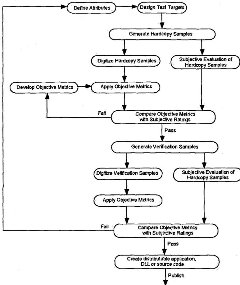
Figure 2. Instrument based metric development procedure
