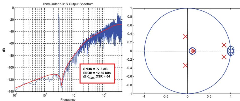
**Figure 6.19:** Simulated output PSD and the NTF pole-zero plot for the third-order CIFF-type KD1S modulator. Here,  $f_s = 100 \text{ MHz}$ ,  $K_{path} = 8$ ,  $f_{s,new} = 800 \text{ MHz}$ ,  $OSR = 8$ , and  $BW = 6.25 \text{ MHz}$ .
