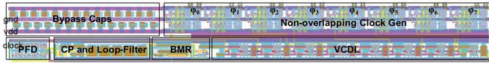
**Figure 7.10:** Layout of the multi-phase clock generator using a DLL designed in 500-nm CMOS process.
