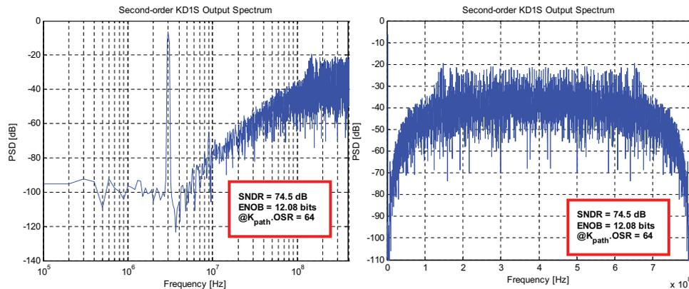
**Figure 6.17:** Spectre simulated spectrum for the second-order KD1S modulator implemented with switched-capacitors and  $f_{un}$  limited op-amp (log and linear frequency axes). Here,  $f_s = 100$  MHz,  $K_{path} = 8$ ,  $f_{s,new} = 800$  MHz,  $OSR = 8$ , and  $BW = 6.25$  MHz.
