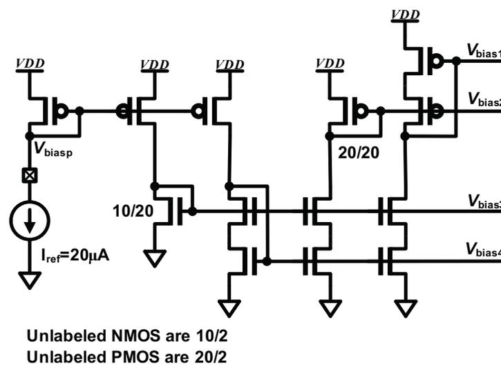
**Figure 7.21:** Bias generation circuit for the op-amps.
