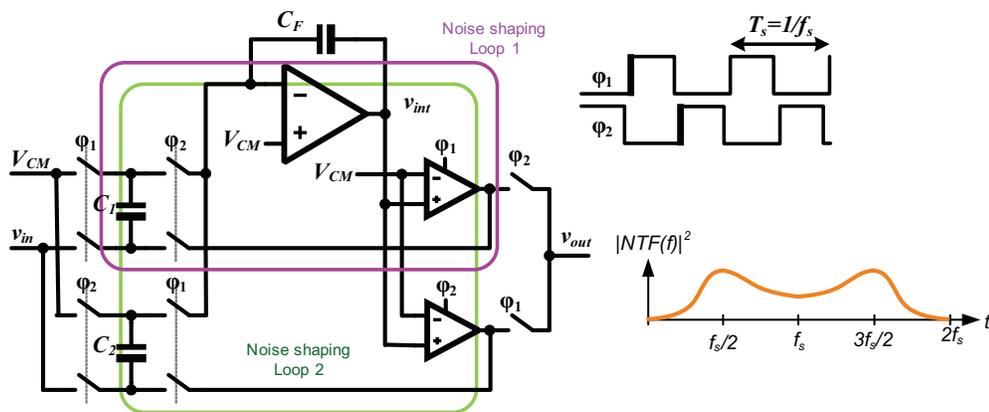
**Figure 3.9:** A first-order delta-sigma modulator employing double-sampling.
