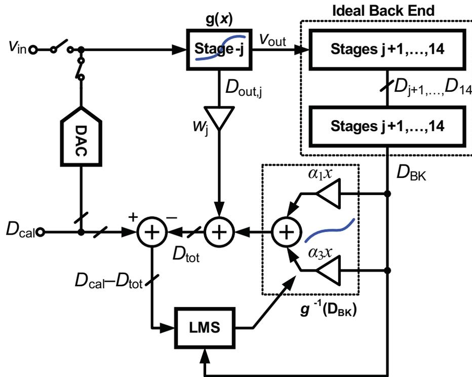
**Figure 3.2:** Diagram showing the concept of digital calibration of a pipelined ADC in [1].
