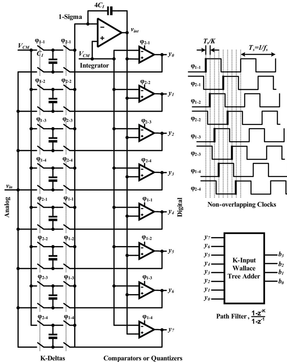
Figure 4.6: The  $K$ -Delta-1-Sigma modulator topology.
