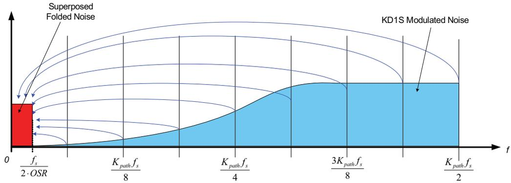
**Figure 4.19:** Noise-folding effects in a KD1S modulator due to path gain mismatches. The shaped quantization noise from the frequencies  $kf_s$ ,  $k = 1, \dots, K_{path}$  gets folded into the signal band.
