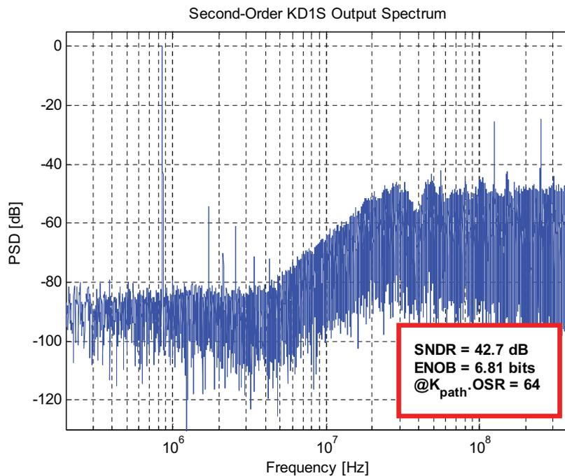
**Figure 7.38:** Measured PSD of the second-order KD1S modulator fabricated in 500-nm CMOS. Here,  $f_{in} = 870$  KHz,  $f_s = 100$  MHz,  $f_{s,new} = 800$  MHz,  $K_{path} = 8$ ,  $K_{path} \cdot OSR = 64$ , and  $BW = 6.25$  MHz.
