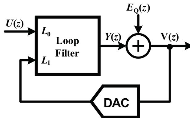
**Figure 6.1:** A generalized structure of a delta-sigma modulator.
