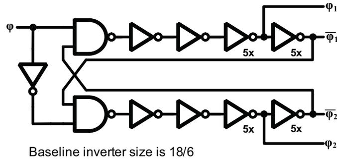
**Figure 7.8:** The non-overlapping clock generator for generating phases  $\phi_1[i]$ ,  $\overline{\phi_1[i]}$ ,  $\phi_2[i]$  and  $\overline{\phi_2[i]}$  from the DLL outputs  $\phi[i]$ , where  $i = 0, 1, \dots, 7$ .
