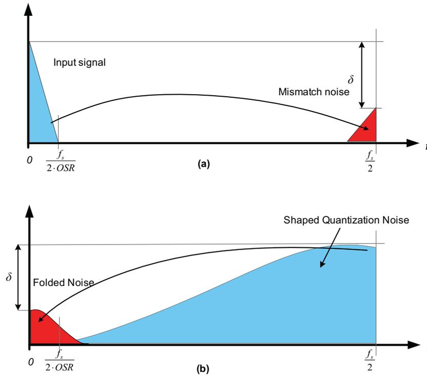
**Figure 3.12:** Noise folding effect due to the path-gain mismatch in a double-sampling DSM. (a) Gain mismatch effect on the input path, (b) Gain mismatch effect on the feedback path where the quantization noise is folded back into the signal band.
