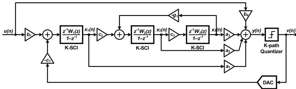
**Figure 6.18:** The synthesized third-order, single-bit CIFF KD1S modulator.
