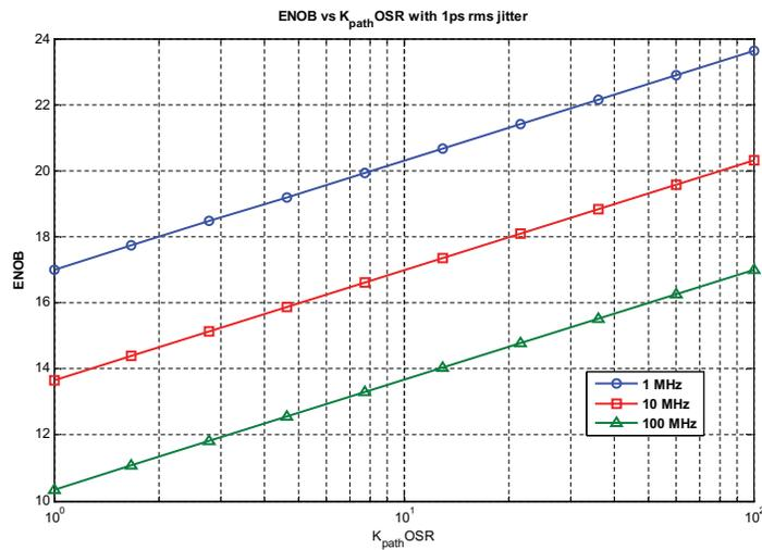
**Figure 4.21:** ENOB vs the effective oversampling ratio for a  $K$ -path sampling scheme with 1 ps rms clock jitter. The plots are for input frequencies ( $f_{in}$ ) of 1 MHz, 10 MHz and 100 MHz. The effective sampling frequency for each of the plots is  $f_{s,new} = 2K_{\text{path}} \cdot \text{OSR} \cdot f_{in}$ .
