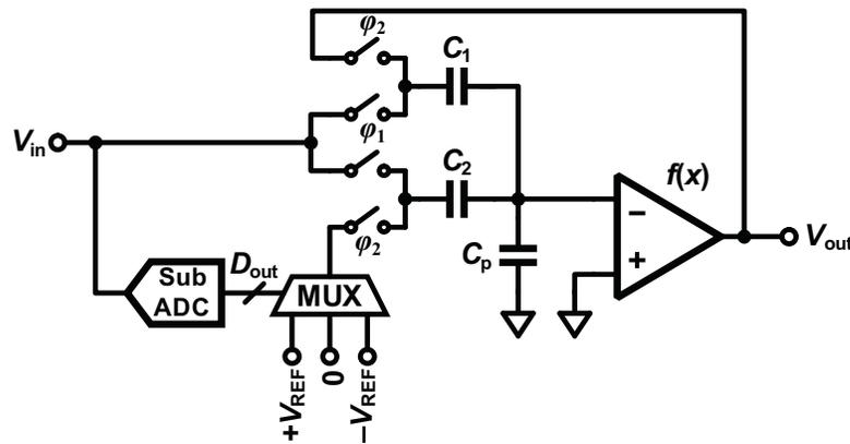
**Figure 3.1:** A 1.5-bit pipelined stage (MDAC) [1].
