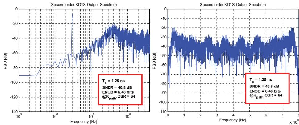
**Figure 5.14:** Spectre simulated PSD (log and linear frequency scales) of the second-order KD1S modulator with comparator delay  $T_c = 1.25\text{ns}$  and the first comparator is clocked on  $\phi_{2-1}$ . Here,  $f_s = 100\text{MHz}$ ,  $K_{path} = 8$ ,  $f_{s,new} = 800\text{MHz}$ ,  $f_{un} = \frac{3}{8}f_{s,new} = 300\text{MHz}$ ,  $OSR = 8$ , and  $BW = 6.25\text{MHz}$ .
