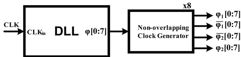
**Figure 7.9:** The complete DLL based multi-phase clock generation circuit .
