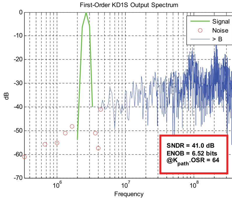
**Figure 7.30:** Simulation results for the first-order KD1S modulator designed in 500-nm CMOS. In these results,  $f_{in} = 2.67$  MHz,  $f_s = 100$  MHz,  $K_{path} = 8$ ,  $f_{s,new} = 800$  MHz,  $K_{path} \cdot OSR = 64$ , and  $BW = 6.25$  MHz.
