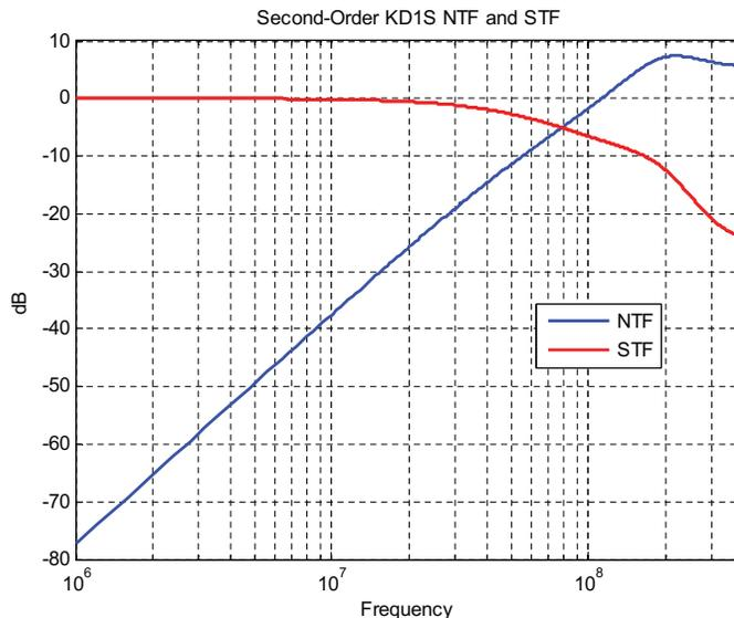
**Figure 5.6:** NTF and STF for the second-order KD1S modulator with  $f_s = 100$  MHz,  $K_{path} = 8$ ,  $f_{s,new} = 800$  MHz,  $f_{un} = \frac{3}{8}f_{s,new} = 300$  MHz,  $OSR = 8$ , and  $T_c = 0$ .
