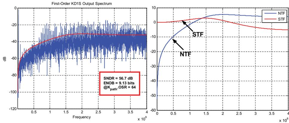
**Figure 4.10:** KD1S noise-shaping with an op-amp with finite unity gain frequency ( $f_{un} = \frac{3}{8}f_{s,new} = 300$  MHz). The second plot shows the NTF and STF for the modulator. Here,  $f_s = 100$  MHz,  $K_{path} = 8$ ,  $f_{s,new} = 800$  MHz,  $OSR = 8$ , and  $BW = 6.25$  MHz.
