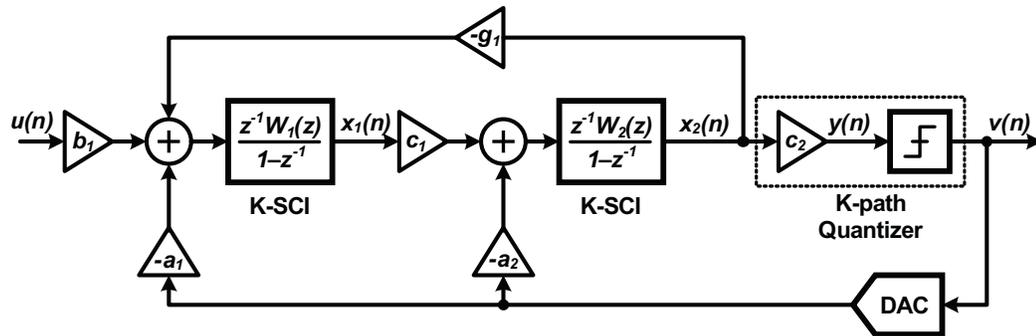
**Figure 6.14:** The synthesized second-order, single-bit, NTF-zero optimized CIFB KD1S modulator.
