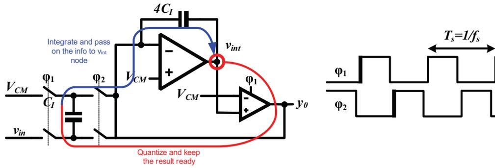
**Figure 3.5:** A first-order discrete-time delta-sigma modulator.
