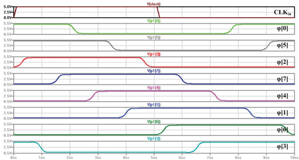
**Figure 7.12:** Eye diagram for the eight clock phases generated from the DLL in the locked condition. Here the input clock frequency is 100 MHz.
