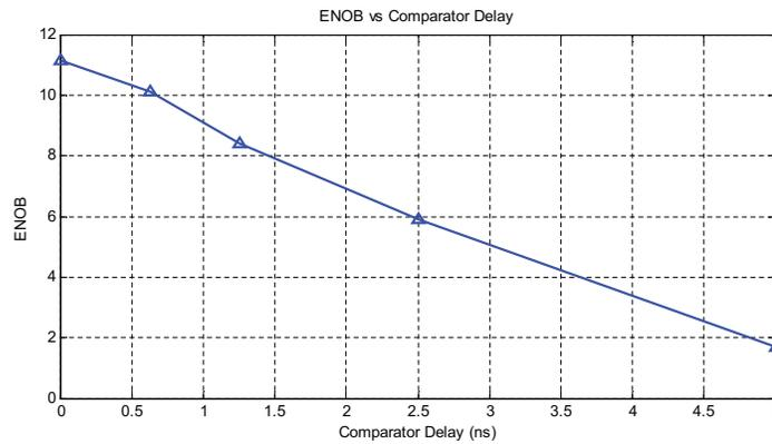
**Figure 5.20:** Effective resolution (ENOB) vs the Comparator delay for the second-order KD1S modulator measured with sinusoidal inputs. Here, the effective clock frequency is  $f_{s,new} = 800$  MHz and  $BW = 6.25$  MHz.
