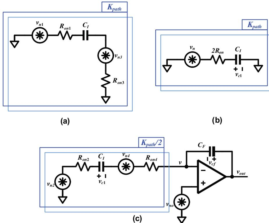
**Figure 4.22:** Noise analysis for the  $K$ -path integrator: (a) Equivalent noise during the sampling phase for each of the capacitors. (b) Equivalent noise schematic for (a). (c) Equivalent noise schematic during the integration phase.
