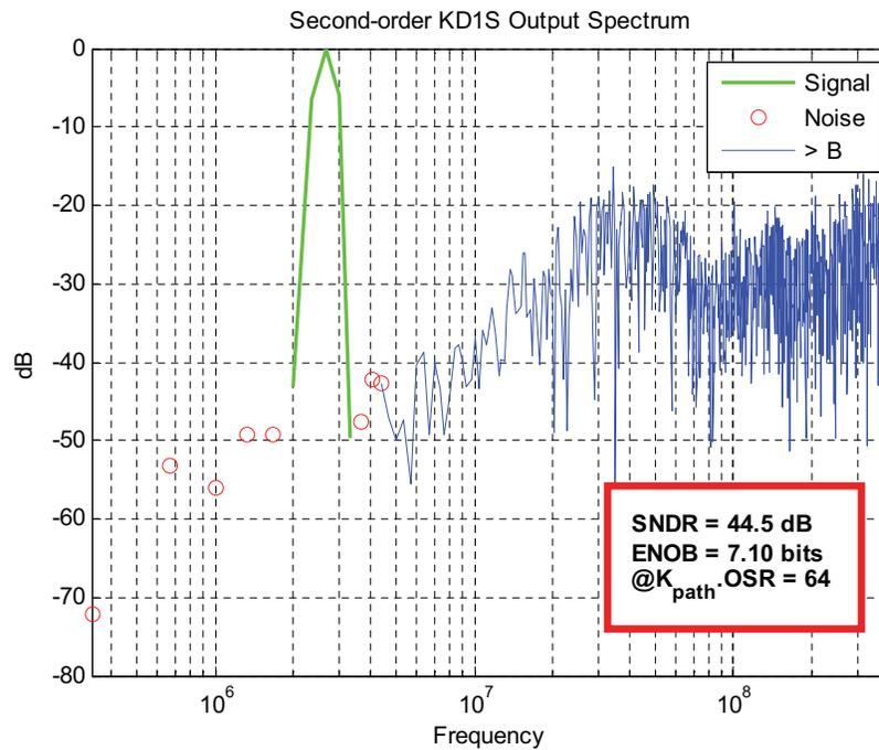
**Figure 7.32:** Simulation results for the second-order KD1S modulator designed in 500-nm CMOS. In these results,  $f_{in} = 2.67$  MHz,  $f_s = 100$  MHz,  $K_{path} = 8$ ,  $f_{s,new} = 800$  MHz,  $K_{path} \cdot OSR = 64$ , and  $BW = 6.25$  MHz.
