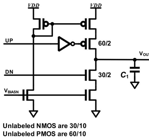
**Figure 7.5:** Charge pump employed in the DLL.
