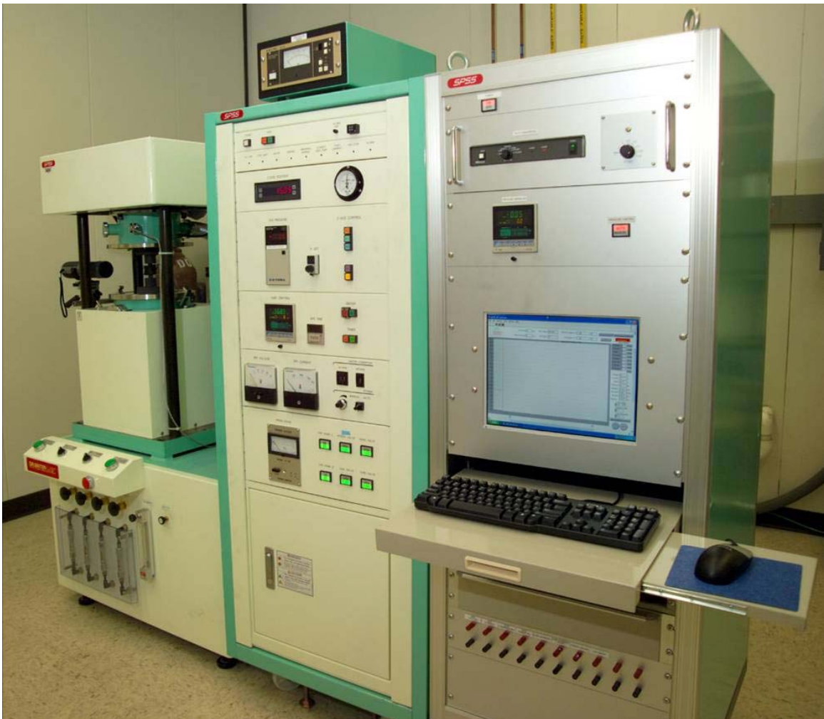
Figure 3.1. Dr. Sinter Lab SPS-515S (SPS Syntex Inc., Kanagawa, Japan) spark plasma sintering machine owned by Boise State University. The process chamber is on the left, the machine controls are on the center unit, and the analysis unit is on the right.
