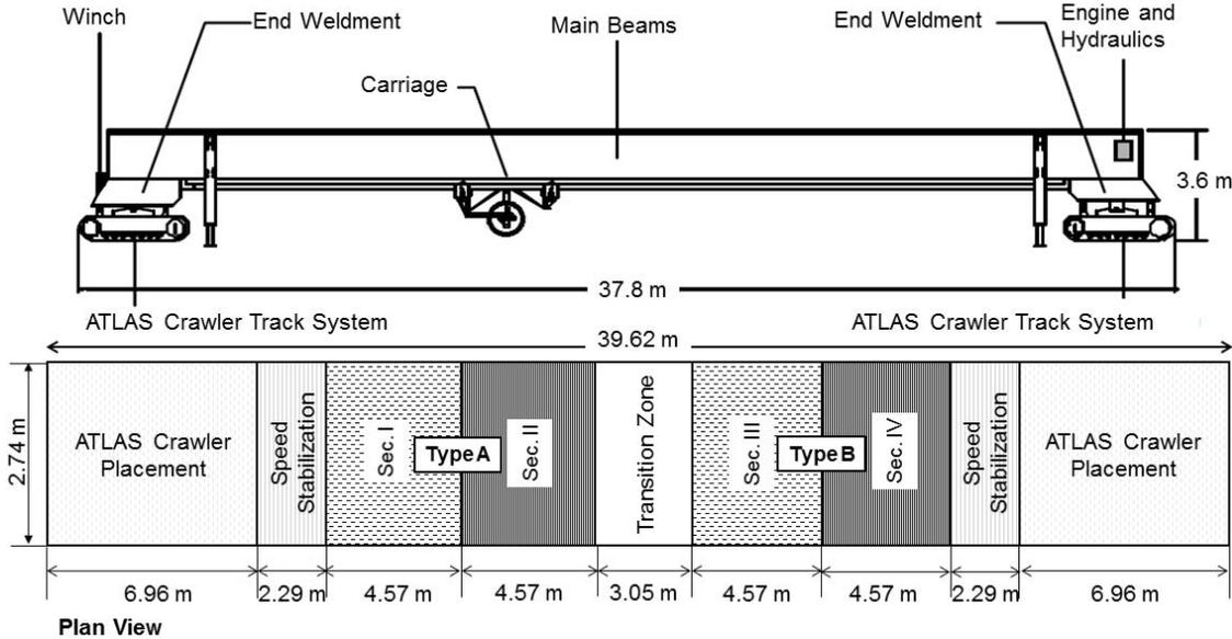
Figure 1: Plan view of the constructed test sections
