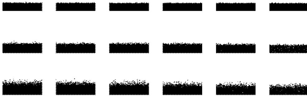
Figure 8. Edge samples for constant raggedness attribute. Top row samples have raggedness = 5; Middle row, raggedness = 10, Bottom row, raggedness = 20.
