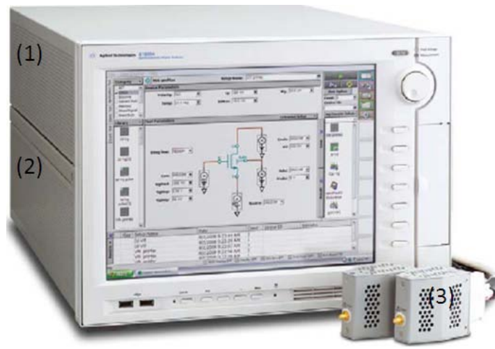
Figure 4.3: Agilent B1500A with RSU units displayed. The Source Monitor Units (1) and B1530A WGF MU (2) are accessed through a panel at the back of the B1500A.
