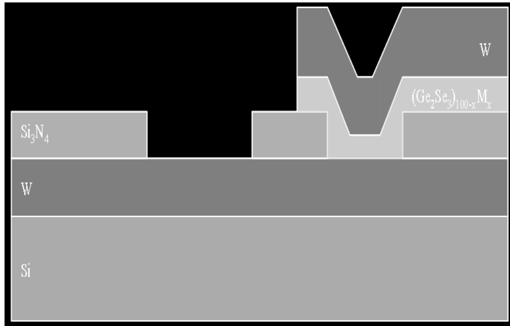
Figure 3.1: Representation of the cross-section for the Ternary devices [24].
