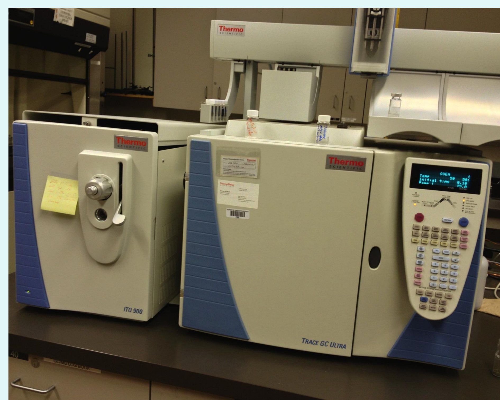
Figure 3. GC-MS instrument used to quantitate and qualitate terpenes
