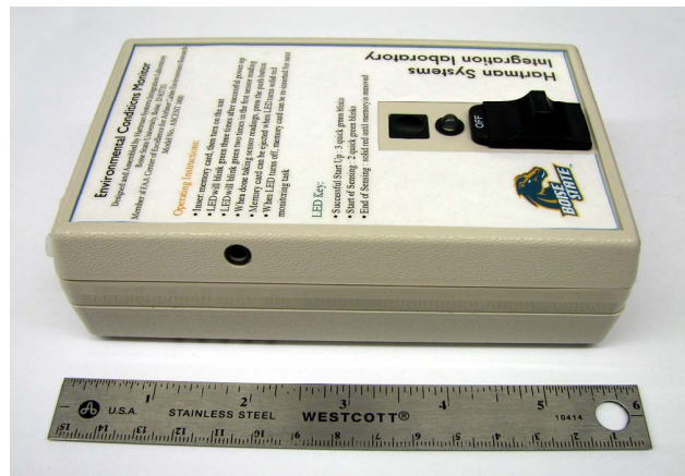
Fig. 4. The sensor module's external form. The sensor module has overall dimensions of 15.3 x 9.2 x 5.4 cm.
