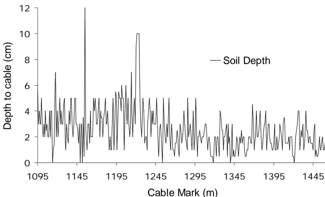
**Figure 3.4. Burial depth for 375 meters of DTS fiber-optic cable used for sampling snow-soil interface temperatures. The cable marks represent measurement locations not absolute distance from the measuring device.**
