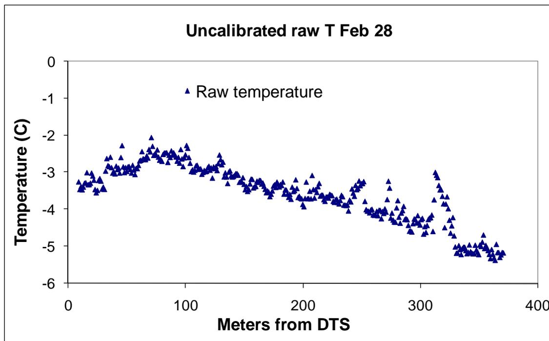
**Figure 3.5. February 28 raw temperature trace (uncalibrated) for 370 meters of cable under uniform conditions and negligible melt. The break in slope represents damage to the cable at the break.**
