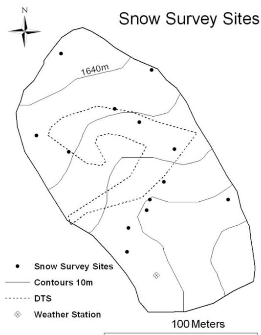
**Figure 3.1. Thirteen points used for weekly snow surveys. The points were chosen to represent redundant sampling for all faces and slopes in the watershed. DTS Fiber optic-cable placement yielding snow-soil interface temperatures.**
