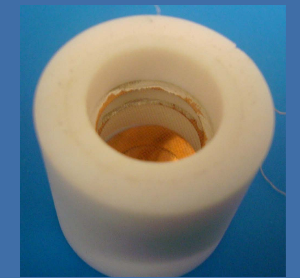
Energy analyzer fabricated using Teflon tubing
