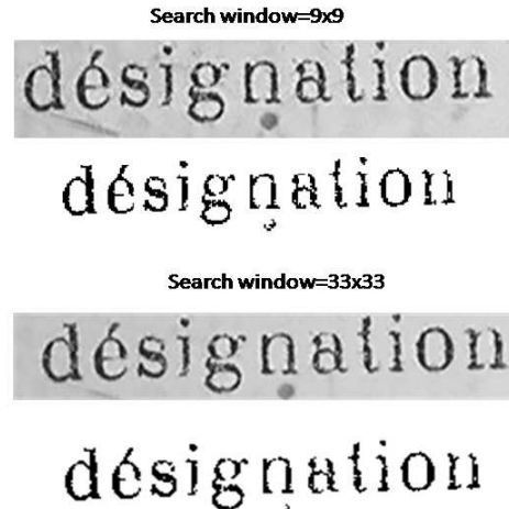
Figure 1. Influence of the size of search window parameter in NLmeans. Filtered and binarized sample word. Large windows regularize more but degrade fading character parts.
