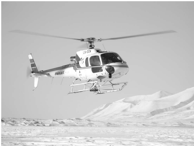
Figure 7. Photograph showing the 1000-MHz shielded antennas suspended from the cargo hook of the helicopter. Photo: D. Dickins.
