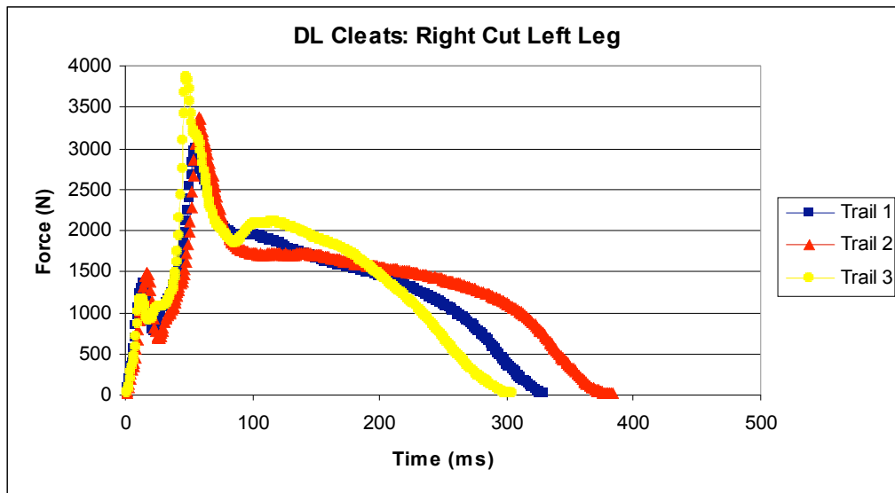
Figure 5: Vertical ground-reaction forces on the left leg with football cleats performing a right cut
