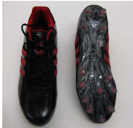
The surface area of each cleated athletic shoe was calculated. The diameter of each stud was measured using Mitutoyo® calipers. The area of the stud was calculated using the following equation:
